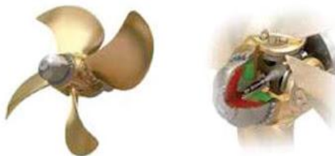
Gambar 2.3.2 Fixed pitch propeller
