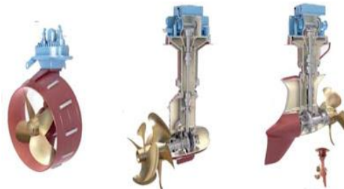
Gambar 2.3.4 Azzimuth thrusters http://www.maritimeworld.web.id/2011/04/macam-macam-jenis-propeller-baling.html
