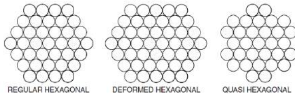
Gambar 2.16 Berbagai macam jenis kabel Parallel-Wire Strand (Gimsing & Georgakis, 2012)
