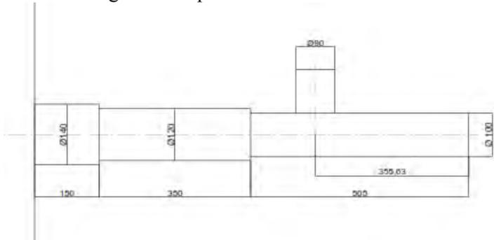
Gambar 3.3 geometri burner
