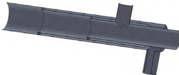
Gambar 1.2 gambar rancangan start up burner potongan samping
