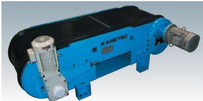
Gambar 4.4 Unit *magnetic separator*
