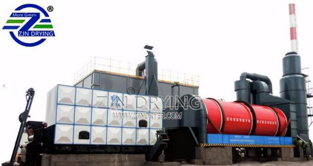
Gambar 4.6 Unit mesin pengering
