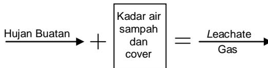
**Gambar 4.34** Skematik *Water Balance*
