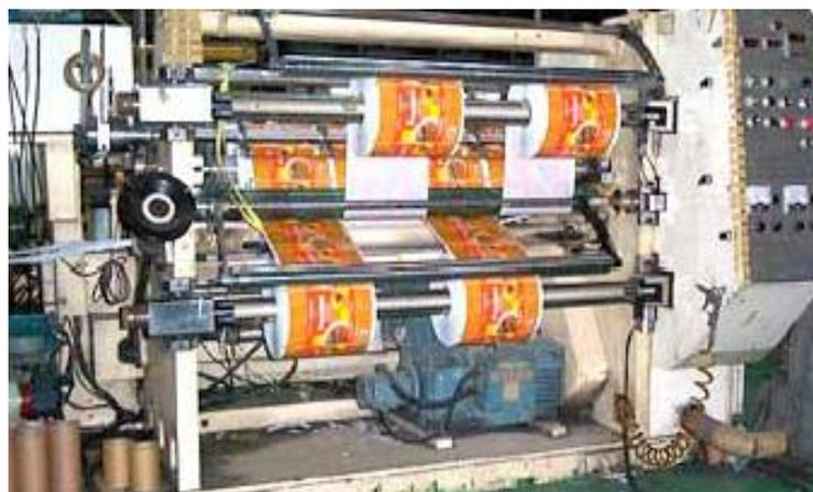
**Gambar 4.13** Mesin *Slitting*
