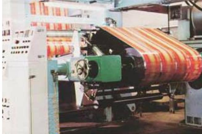
**Gambar 4.10** Mesin *Dry Laminating*
