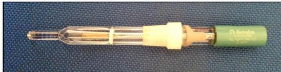
**Gambar 3.8** Elektrode AgCl
