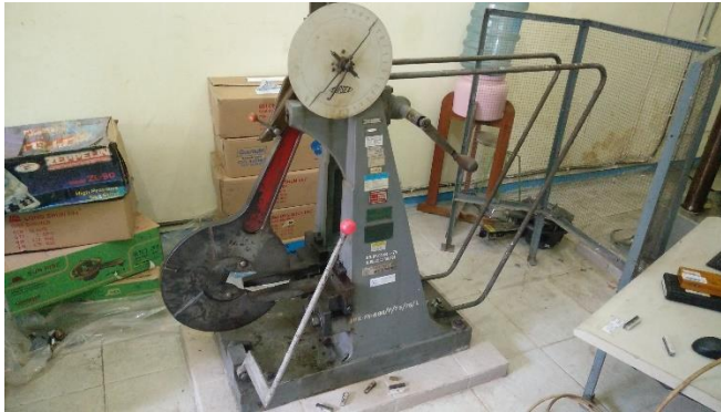
Gambar IV.18. Alat uji impact charpy Baristand.
