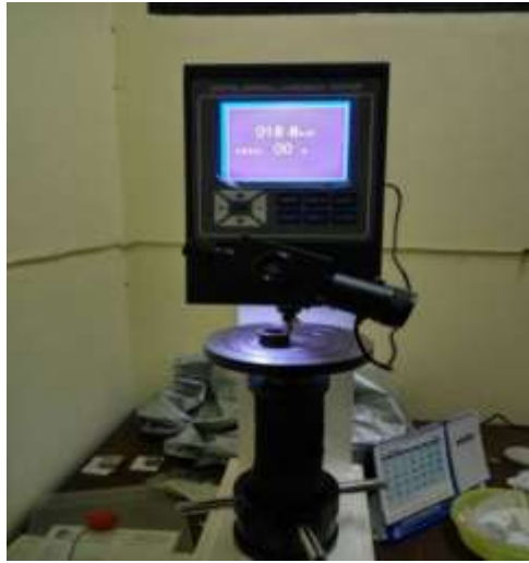
Gambar 3.29 Alat uji kekerasan Digital Brinell Hardness Test
