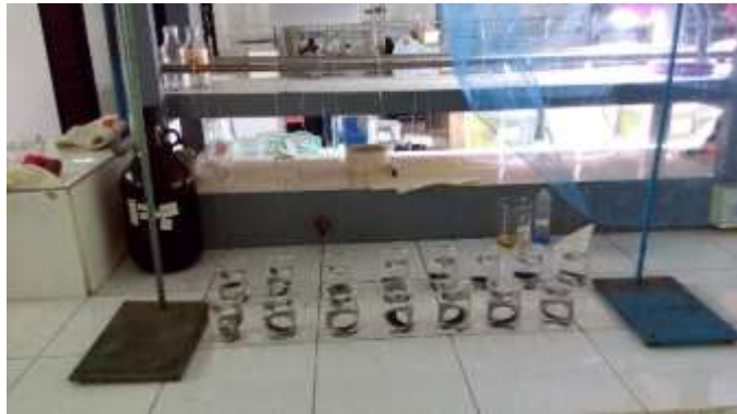
Gambar 4.6 proses pengujian immersion corrosion test
