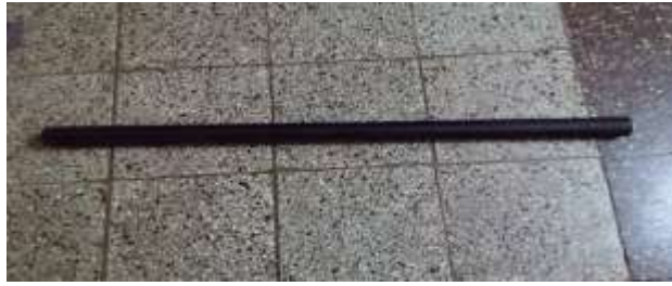
Gambar 3.19 Material Pipa Baja API 5L Grade B
