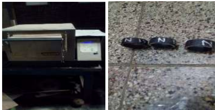
(i) (ii) Gambar 3.25 (i) Furnace, (ii) material hasil Normalising
