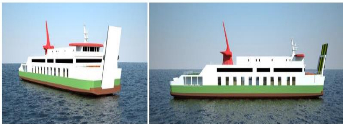
Figure 4.4 Modification of ramp door[12]
