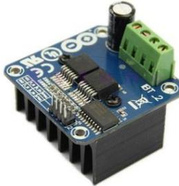
**Gambar 2.6** *Driver* motor BTS7960
