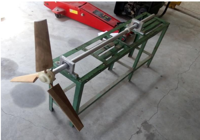
Gambar 2.14 Turbin Angin Sumbu Horizontal 3 Blade Airfoil Clark-Y Model Taper Linear
