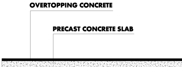
Figure 3.11. Condition of slab precast element before monolith condition (source: Private Documentation)
