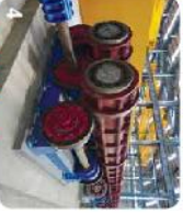
PILE SPINNING The pile is then subjected to air centrifugal force. The pile is spun in a single operation. This ensures uniformity of stress in all the PC bars and hence straightness of the pile.
