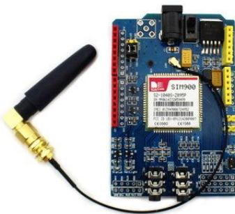
Gambar 2.1 Modul GSM SIM 900L
