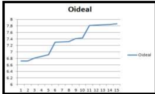
Gambar 4.4 Grafik Linearitas sensor Pressure Transmitter TPS 20-G28P2
