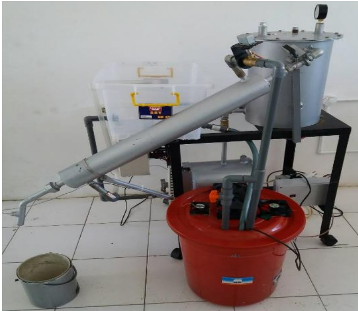
Gambar 3.4 Plant Fluidized Bed Reactor
