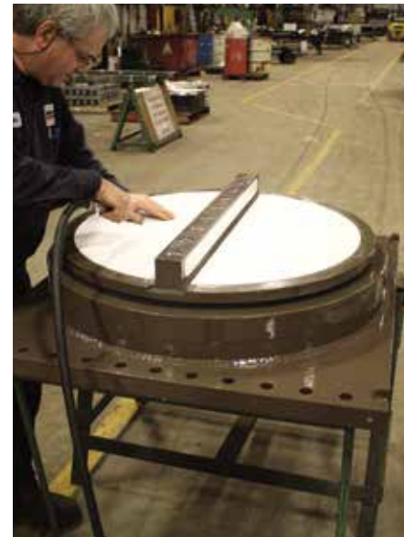
The PTFE disc is cleaned before the silicon lubricant is applied.
