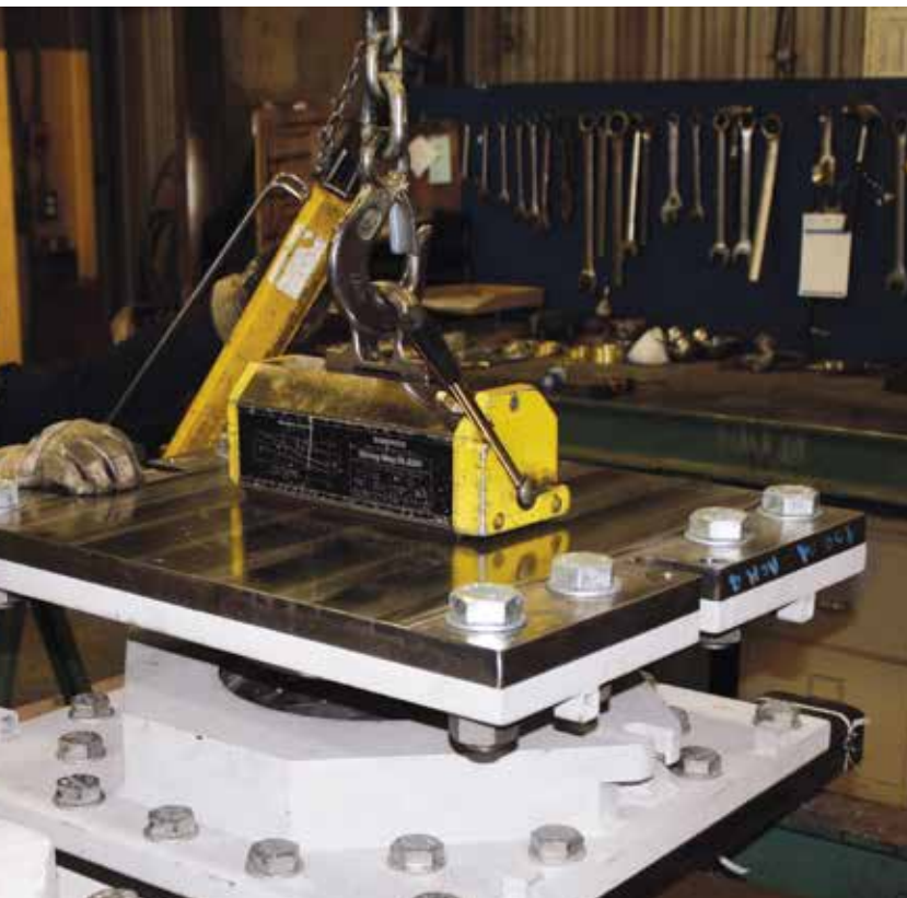
PF Series fixed pot bearing assembly with uplift restraint device
