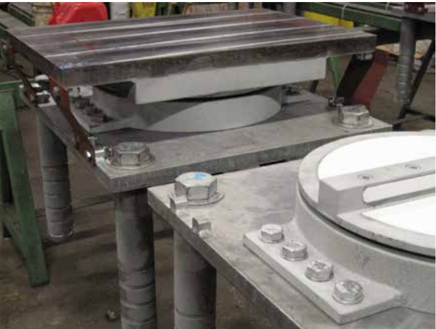
Goodco Z-Tech manufactured 80 pot bearings – PF Series fixed, PM Series multidirectional and PMCG Series unidirectional – for the five-lane Athabasca River Bridge.
