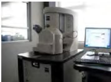
Gambar 3.10 *Scanning Electron Microscope* Zeiss EVO MA 10.
