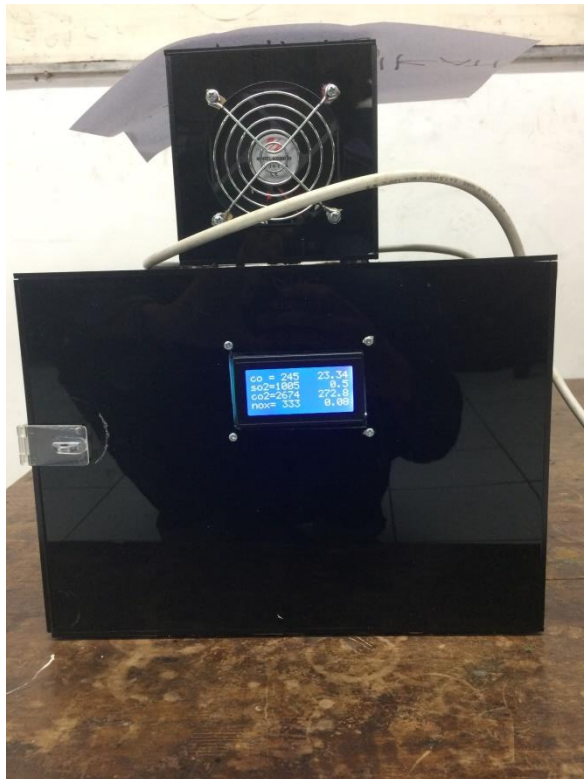
Gambar 4.1 Detector Emission Gass NO x Plant
