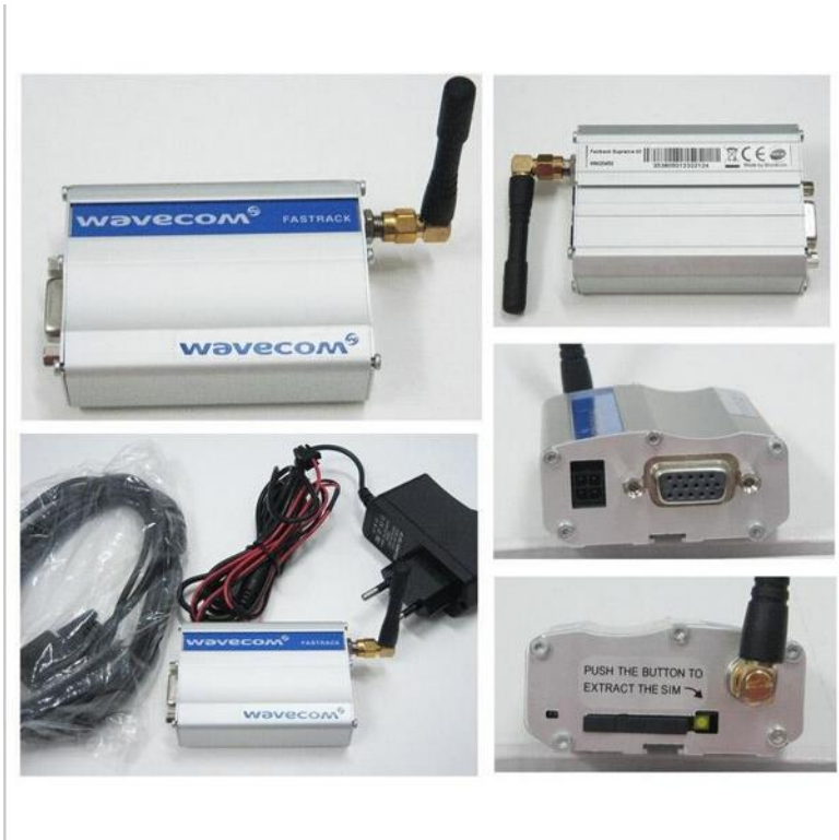
Gambar 2.9 Modem Wavecom Fastrack M1306B Serial
