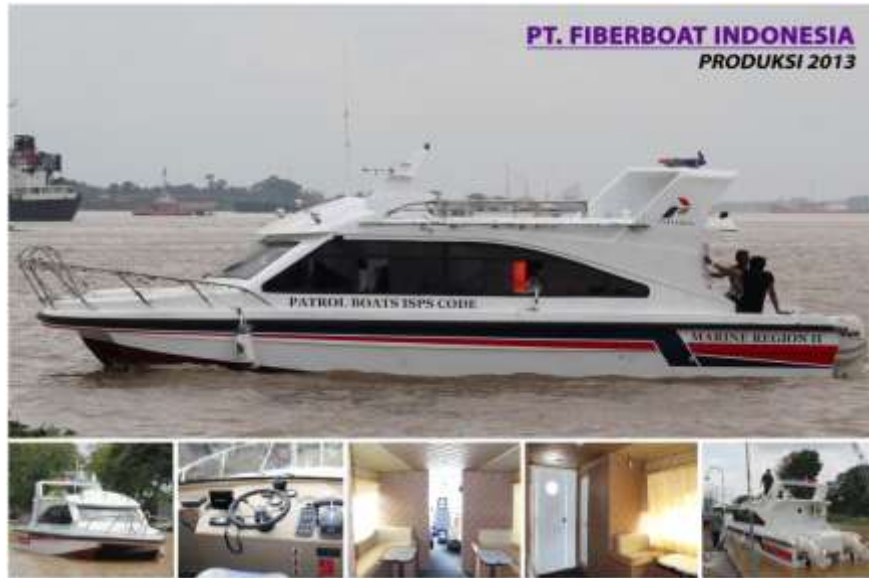
Gambar III. 2 Kapal Patroli katamaran seri FBI.1032.XA (PT.FIBERBOAT INDONESIA,2013)
