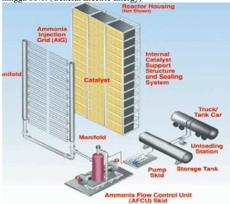
Gambar 2.13 Skema sistem SCR (General Electric Energy)
