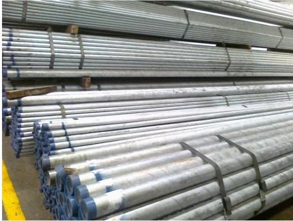
Gambar 2.3 Pipa Galvanized
