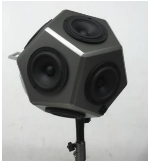
Gambar 4. 1 Purwarupa Vibrastics dodecahedron dengan 12 buah driver speaker SB Acoustics.
