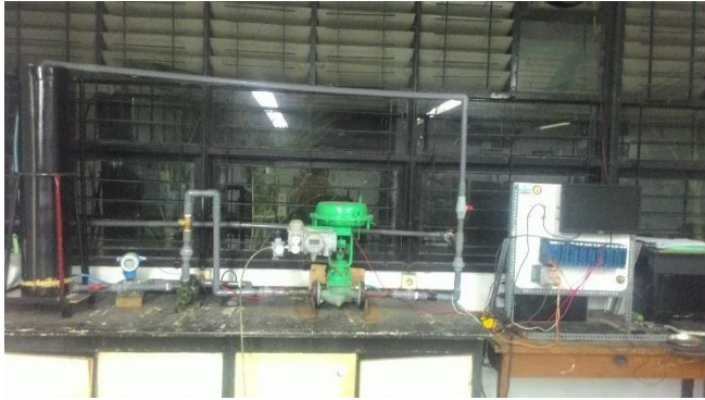
Gambar 3. 4 Plant level real plant
