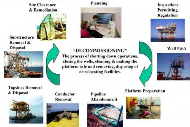
Figure 3 – The Decommissioning Process (TSB Offshore, Inc.)
