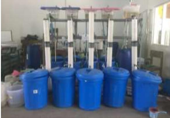
**Gambar 3.2** Reaktor Downflow slow sand filter
