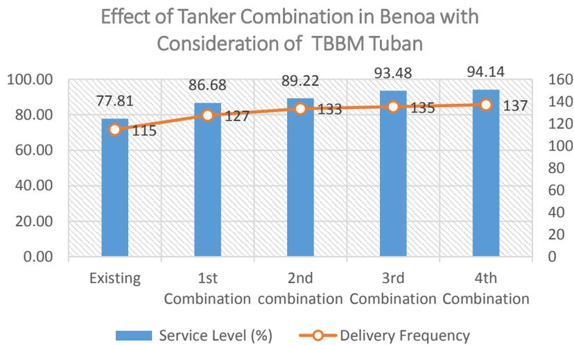
Figure 6. 4 Effect of Tanker Combination to Service Level and Delivery Frequency in *Scenario 2*
