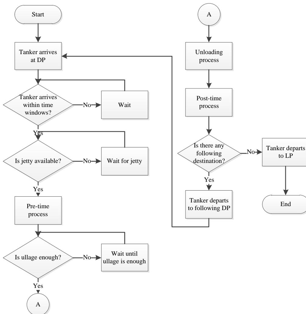
Figure 5. 6 Conceptual Model of Unloading Mechanism
