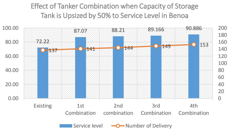
Figure 6. 10 Effect of Upsizing Storage Tank Capacity to Service Level in Benoa
