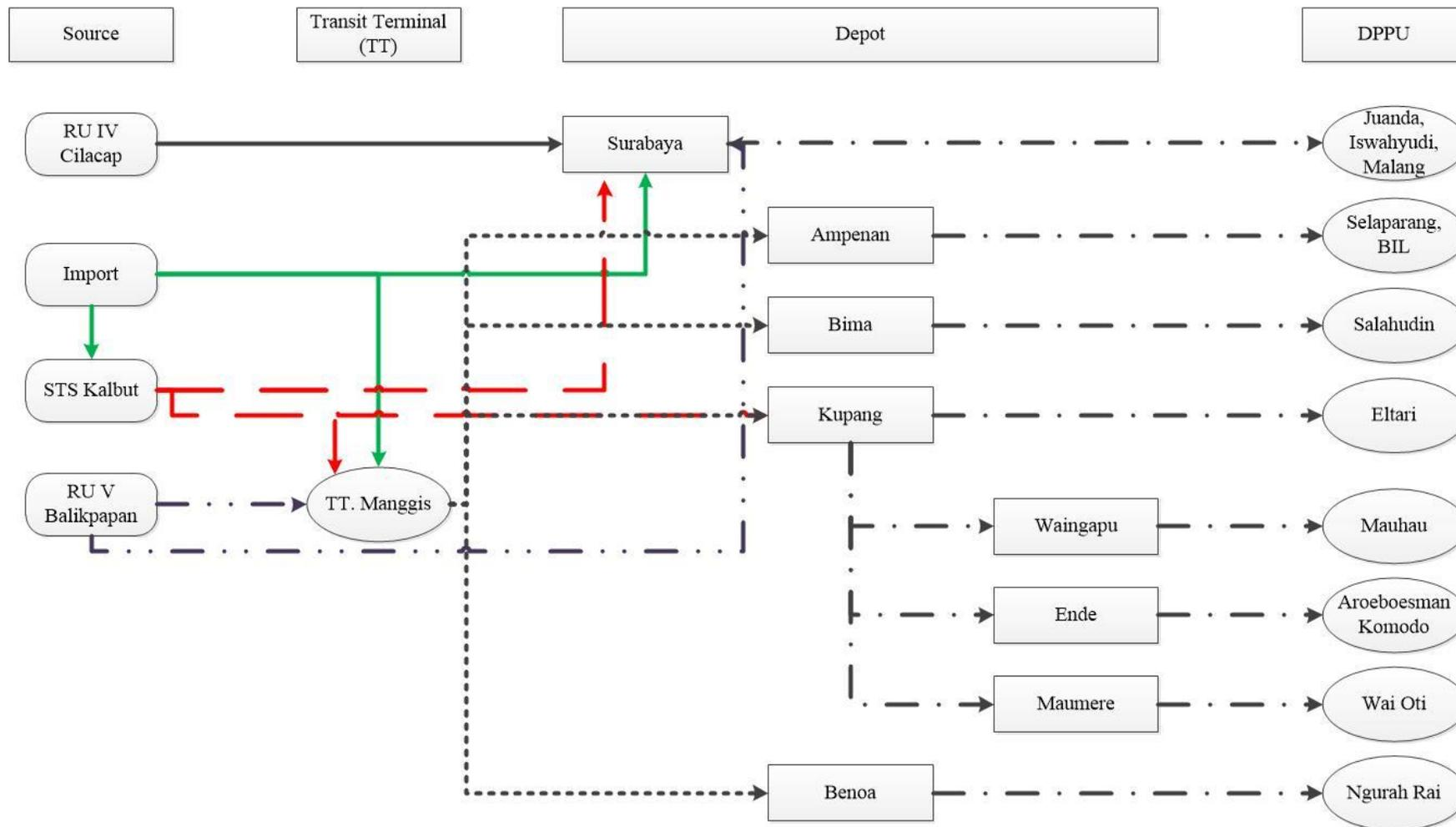
Figure 2. 4 The Supply and Distribution Pattern of Avtur in MOR V during Regular Condition (Pertamina, 2017)
