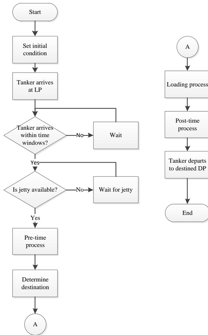
Figure 5. 3 Conceptual Model for Loading Mechanism
