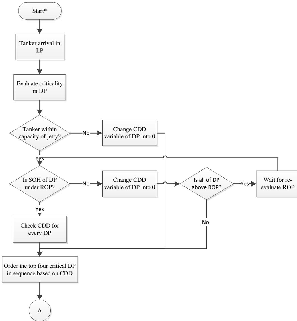
Figure 5. 4 Conceptual Model for Selecting Discharge Port
