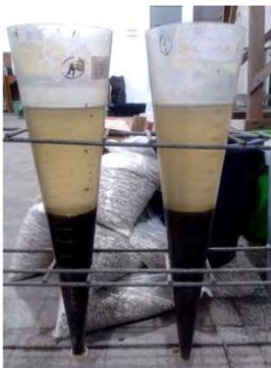
**Gambar 4. 2 *Settleability Solid Test***
