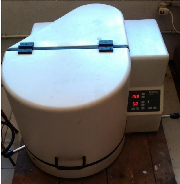
Gambar 3. 1 *Planetary ball mill*.
