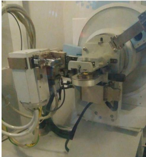
Gambar 3. 2 *X-ray Diffractometer.*
