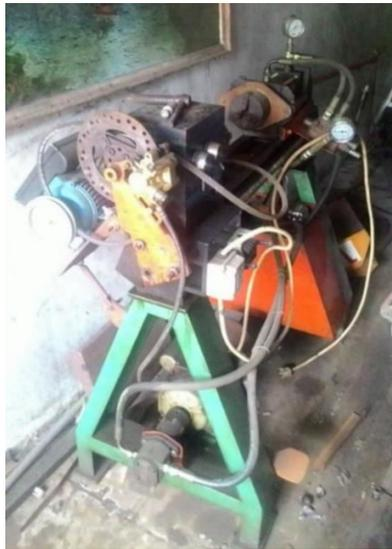
**Gambar 3.3** Mesin *Direct-drive friction welding*
