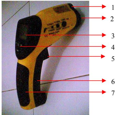
**Gambar 3.6** *Sensor Infrared Sensor Temperature*
