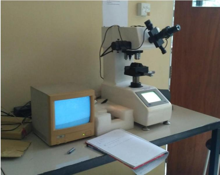
**Gambar 3. 8** Microhardness Vickers Tester
