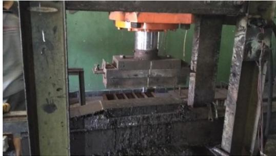
**Gambar 3. 5** Mesin Press kampas rem
