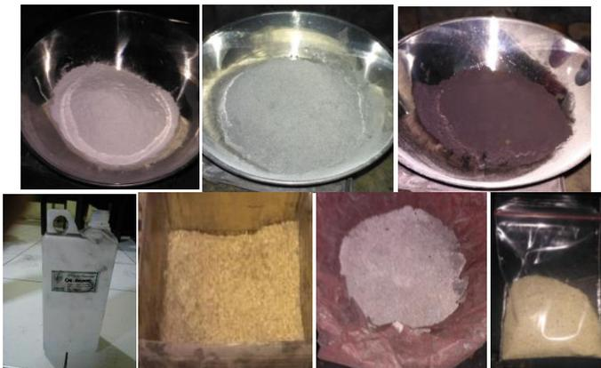
**Gambar 3. 2** Bahan dasar. Dari kiri Aluminium Oxide, Aluminium Powder, Iron Powder, Resin, Waru, Keramik Fiber, dan Pasir Silika
