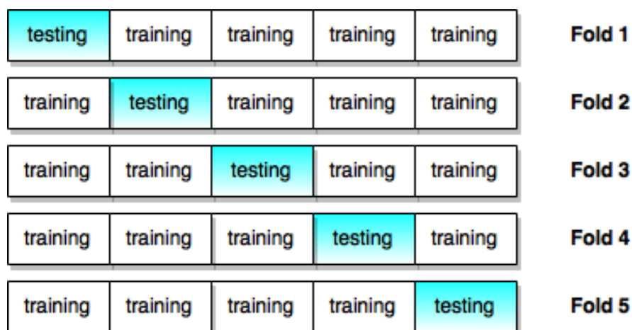
Gambar 2.1 Ilustrasi K-Fold Validation
