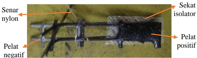
**Gambar 4.1** Susunan spesimen uji 8 Channel Battery Analyzer.
