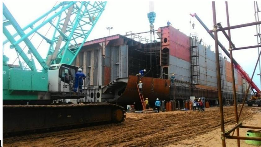
Gambar 5.14 Proses Erection
