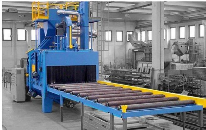
Gambar 5.39. *Shot Blasting & Priming Machine*
