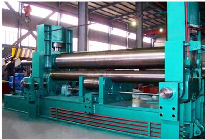
Gambar 5.44. *Plate Bending Machine*
