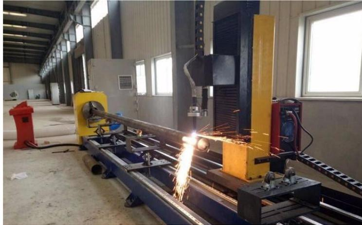
Gambar 5.46. CNC *Plasma Cutting Machine (Pipe)*
