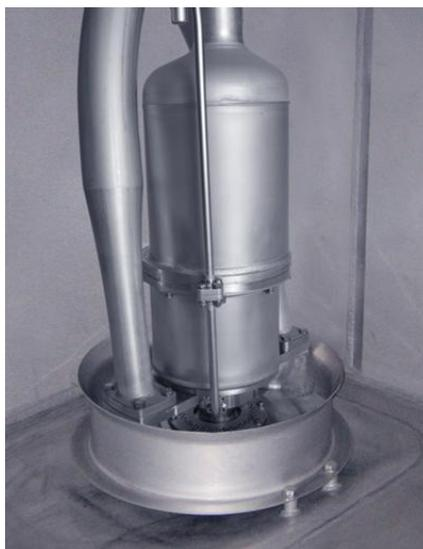
Gambar 5.28. *Submerged Cargo Pump*
