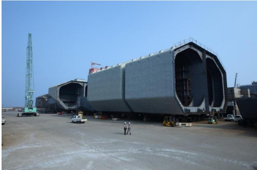
Gambar 2.19. *Independent Tanks Type A (Prismatic Tanks)*
