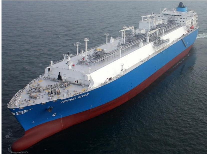
Gambar 2.31. LNG Carrier (*Membrane Tanks*)
