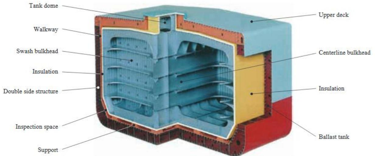
Gambar 2.24. *Cargo Containment Systems Prismatic Tanks* (IHI SPB)
