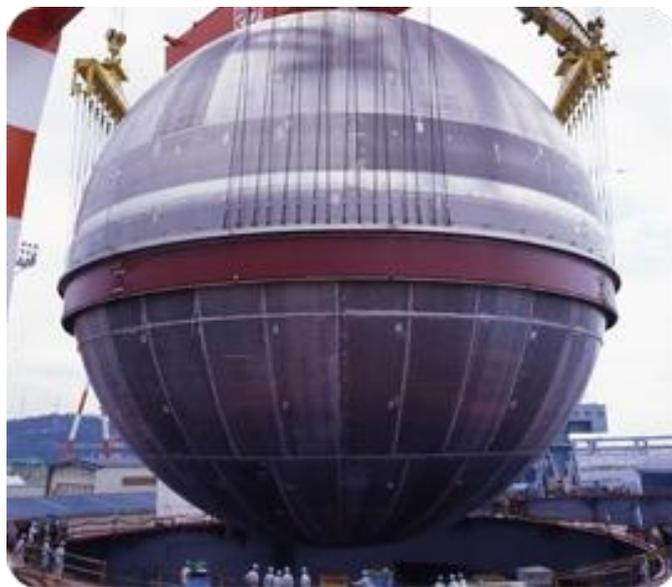
Gambar 2.23. *Spherical Tanks* (Moss)
