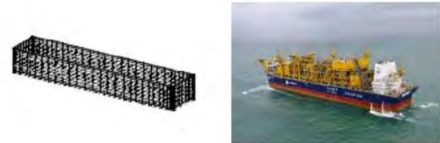
Gambar 2.4.5 *Simple Box* (Conventional Barge)
