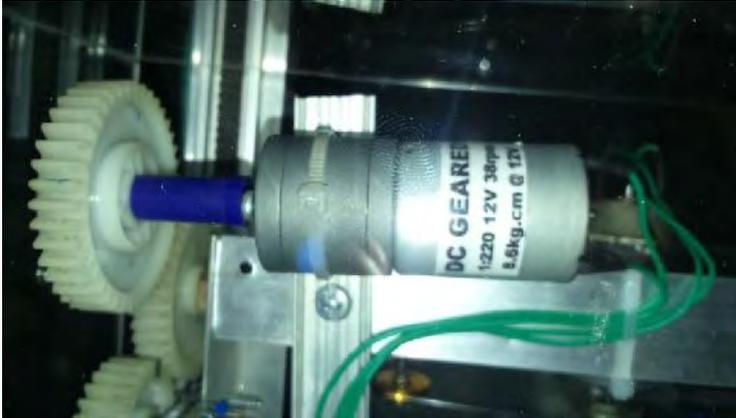
Gambar 2.11 Struktur Eksternal Geared Motor DC
