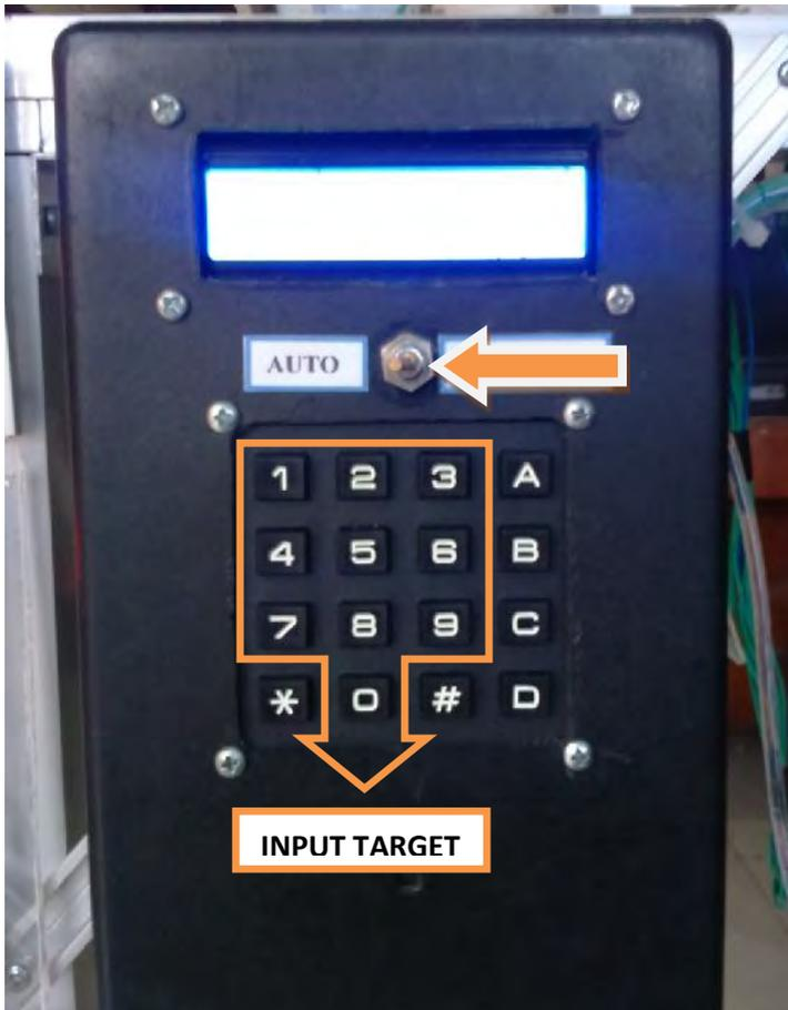
Gambar 4.36 Tombol Perintah Input Target Pada Mode Auto
