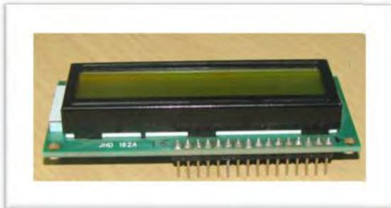
Gambar 2.8 LCD (Liquid Crystal Display)
