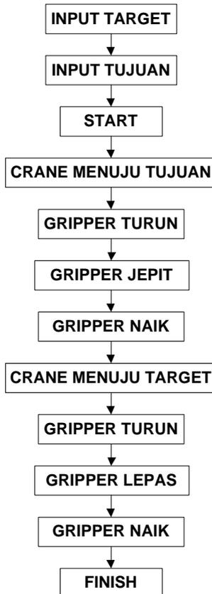
Gambar 4.35 Blok Diagram Alur Pengoperasian Mode Auto
