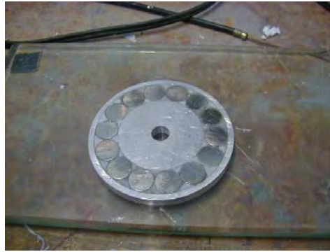
Gambar 2.6 Rotor Motor Listrik Axial ( endless-sphere.com )
