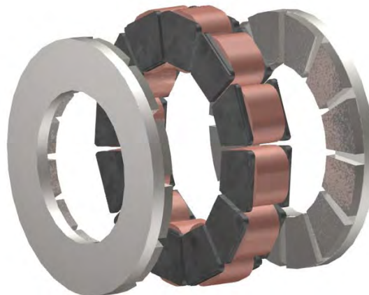
Gambar 2.4 The axial flux motor design ( www.endles-sphere.com )
