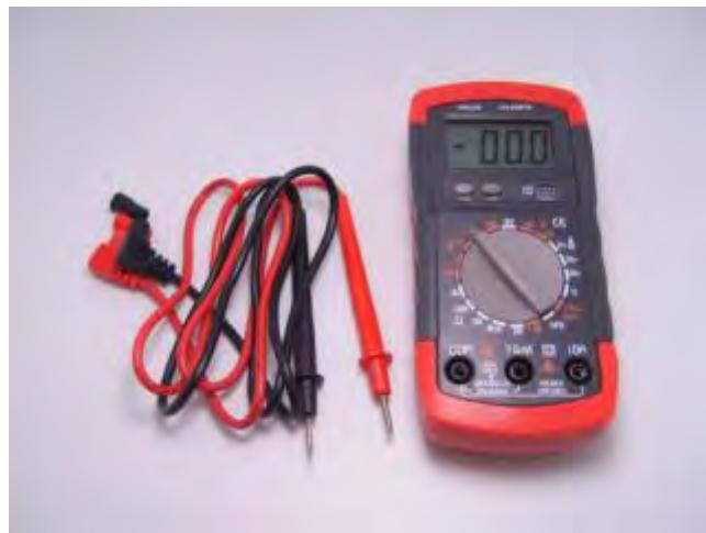
Gambar 3.17 Multimeter digital Heles UX838
