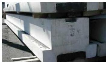
**Gambar 2. 7 Inverted Tee Beam**
