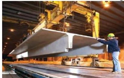
**Gambar 2. 4 Double Tee slab**
