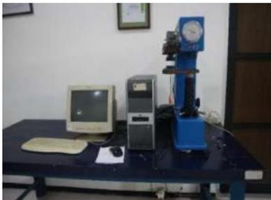
**Gambar 3. 6** Universal Hardness Tester HBRV 187.5A
