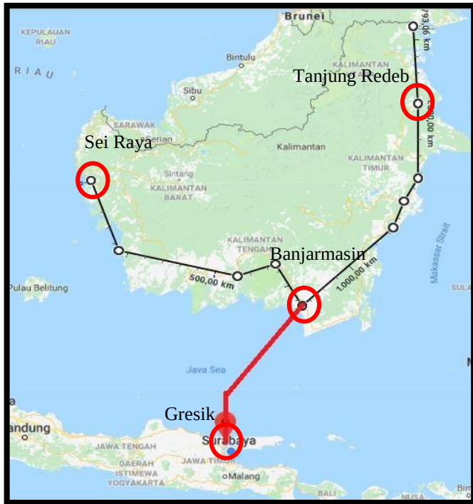
Gambar 3.2. Jalur backbone 500 kV DC
