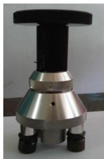
**Gambar 3.3. Elcometer model 106 adhesion tester scale 1**
