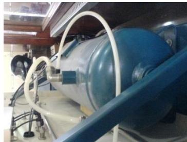
Gambar 2.12 Air receiver Pressure Process Rig 38-714
