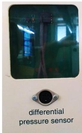
Gambar 2.11 *Differential pressure sensor Pressure Process Rig 38-714*
