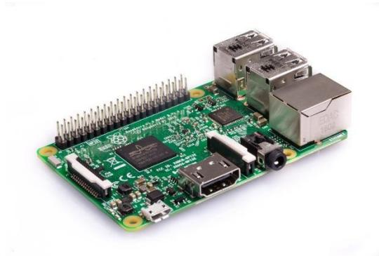
**Gambar 2.3 Raspberry Pi 3 Model B [10]**
