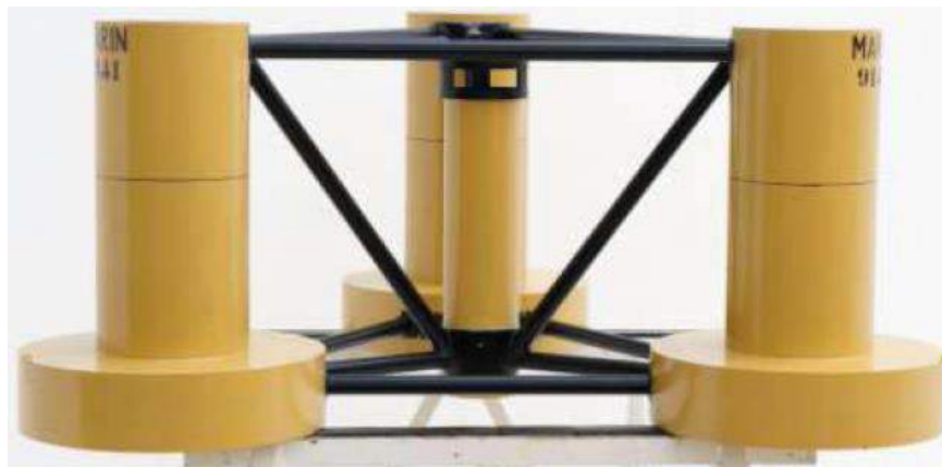
Gambar 3. 4 Model DeepCWind Semisubmersible (NREL, 2014)
