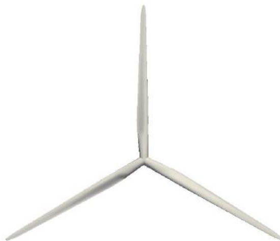
Gambar 3. 2 Model Turbin NREL 5MW Baseline (NREL, 2009)
