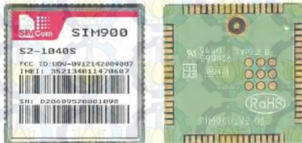
Figure 39: Top view of the SIM900
