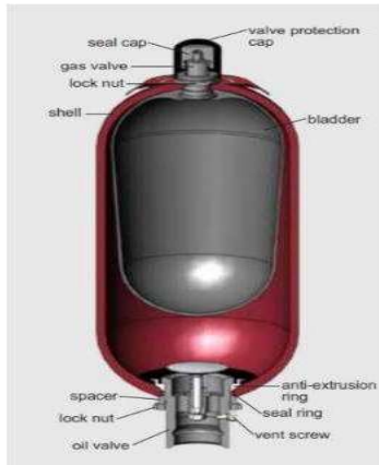
Gambar 2.4 Bladder Accumulator [1]
