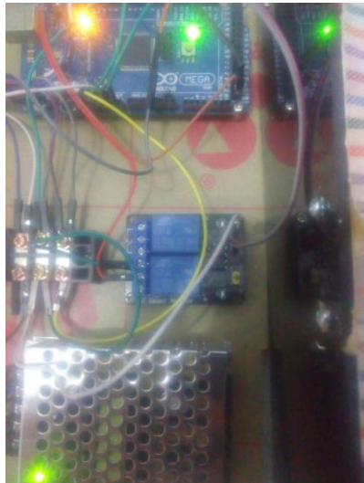
Gambar 4.12 Relay mati saat nilai suhu melebihi threshold
