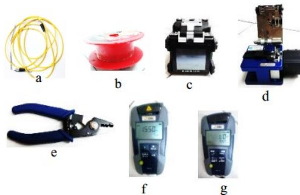
Gambar 3.2 (a) Serat optik *singlemode* SMF-28 step index core 4.2  $\mu\text{m}$  (b) Serat optik *multimode coreless* (c) *Fusion Splicer* (d) *Fiber cleaver* (e) *Fiber stripper* (f) *Optical Light Source* (g) *Optical Power Meter*
